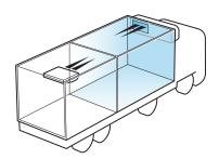
Multiline 8MT is 1100 mm wide and can be mounted in several places. A suitable solution for a movable partition that divides the box crosswise.
