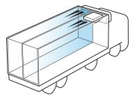
Multiline 7MTL is a slim unit - only 800 mm wide (one pallet width). It can be fitted in a refrigeration corridor both at the front and the rear.
